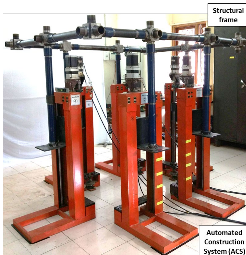
Figure 5.4 Partially constructed structural frame on the Automated Construction System (before instrumentation)
