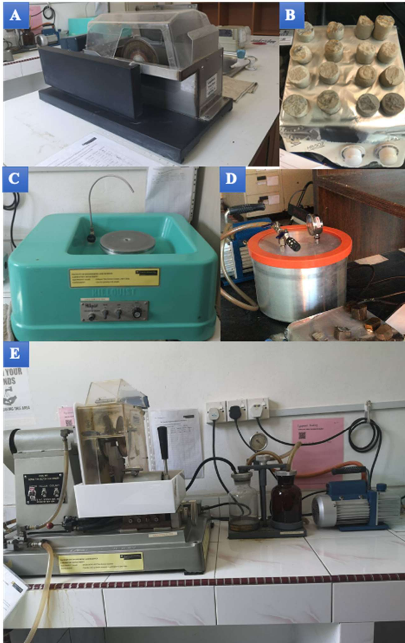
Figure 3.3 Images of A. Lapidary trim saw, B. Hot plate, C. Hillquist thin section grinder, D. Vacuum pot and E. Ingram ward thin section machine.
