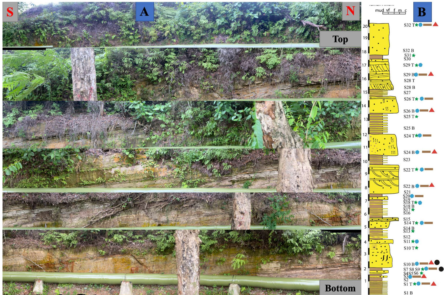
Figure 4.5 Image of A.Taman Awam outcrop, Images are stacked from bottom to top bed, length of the outcrop is about 100m with a thickness of 22m. B. stratigraphic log section showing the location of samples collected
