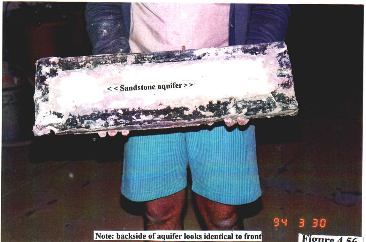
b) Isolated Aquifer after Dismantling
