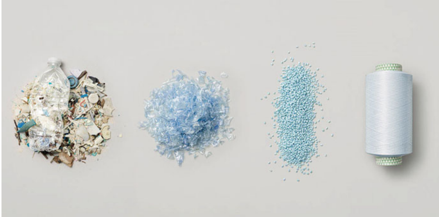
Fig. 3 Converting ocean plastic into yarn. (Parley (2018), with permission)
