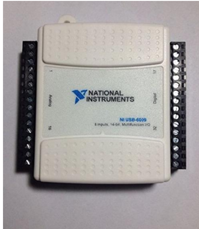
Figure 3-9: Picture of National Instrument Data Acquisition System in flow loop test facility
