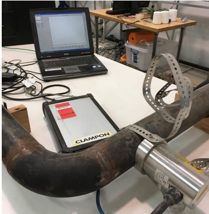
Figure 3-6: Image of ASD, receiving Unit and the Laptop for the Clamp-On ASD used in Flow loop test facility
