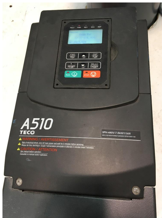
Figure 3-4: Picture of the Variable Speed Drive (VSD) used in flow loop test facility
