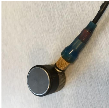
Figure 4-2: A picture of the 1/2 inch diameter Olympus ultrasonic sensor used in this research
