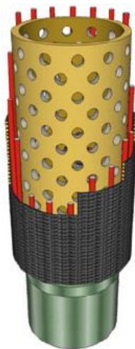
Figure 2-6: Typical make-up of a wire wrapped sand screen [26]
