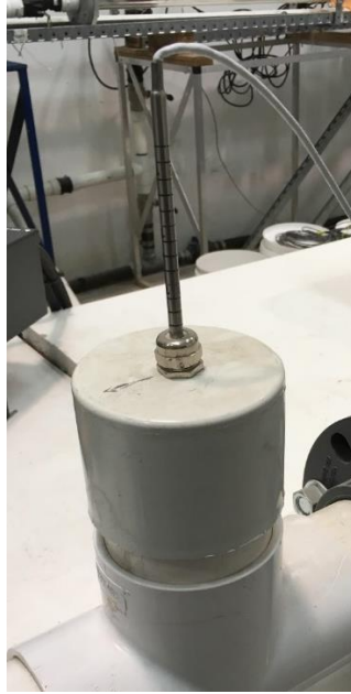
Figure 3-7: Picture of velocity/temperature sensor in flow loop test facility
