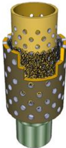
Figure 2-8: Typical make-up of wool wrapped screen [26]
