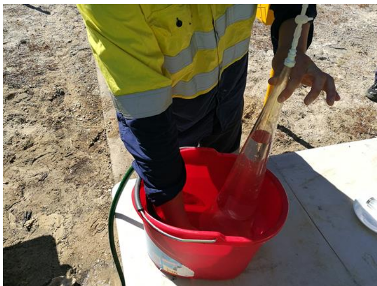
Figure 10 Volumetric flask used to measure the gas separating from the chlorinated water produced by the pilot unit.
