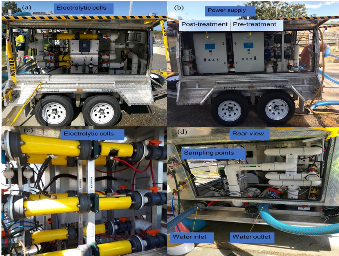
Figure 5 Pilot unit depicting the electrolytic cells (a, c), power supply for the pre- and post-treatment cells (b), the water inlet and outlet and the sampling points (d).
