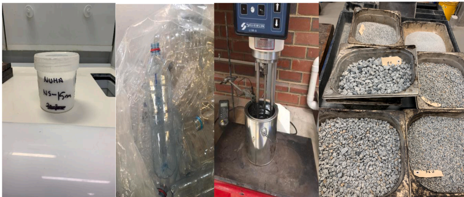
Fig. 2. Materials used in the study (nano-silica, waste plastic, bitumen binder, and granite aggregate, from left to right).
