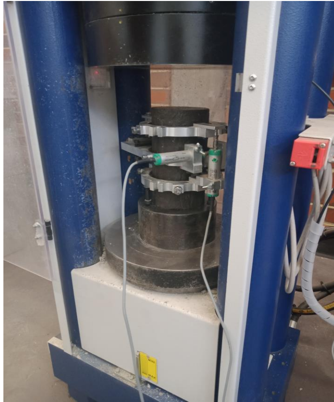
Figure 4.28: Non-destructive lab test conducted for the polymer composite at 28 days to obtain Poisson's ratio and modulus of elasticity
