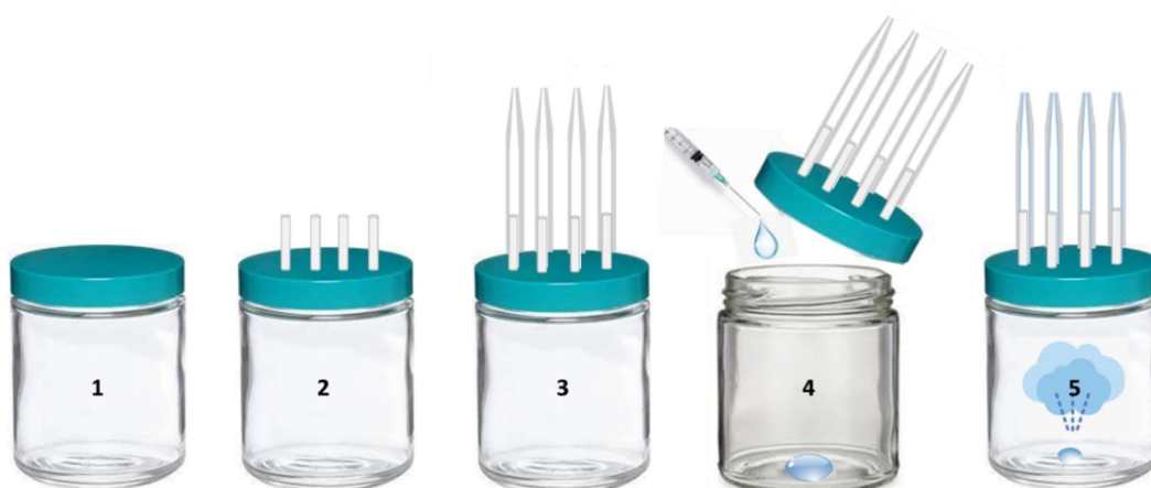
Figure 2.2.5.3: Schematic presentation of silanization process of pipette. (1) glass jar with PTFE (Teflon) cap (2) the caps are joined with tubes (3) pipettes fitted in the tube (4) 1/2 drops of chlorotrimethylsilan added into the jar (5) vapour of the chlorotrimethylsilan goes through the pipettes and makes silanization on the inner surface of the pipettes.
