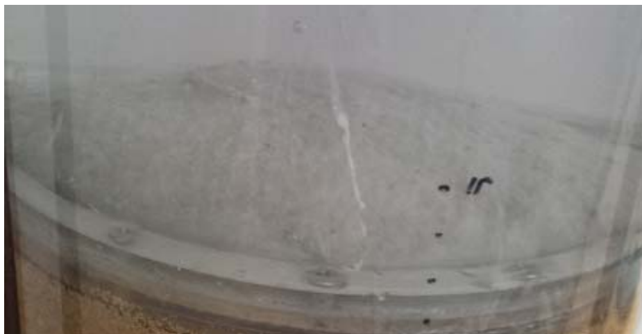
Figure 4.13 GCL starting to be lifted
