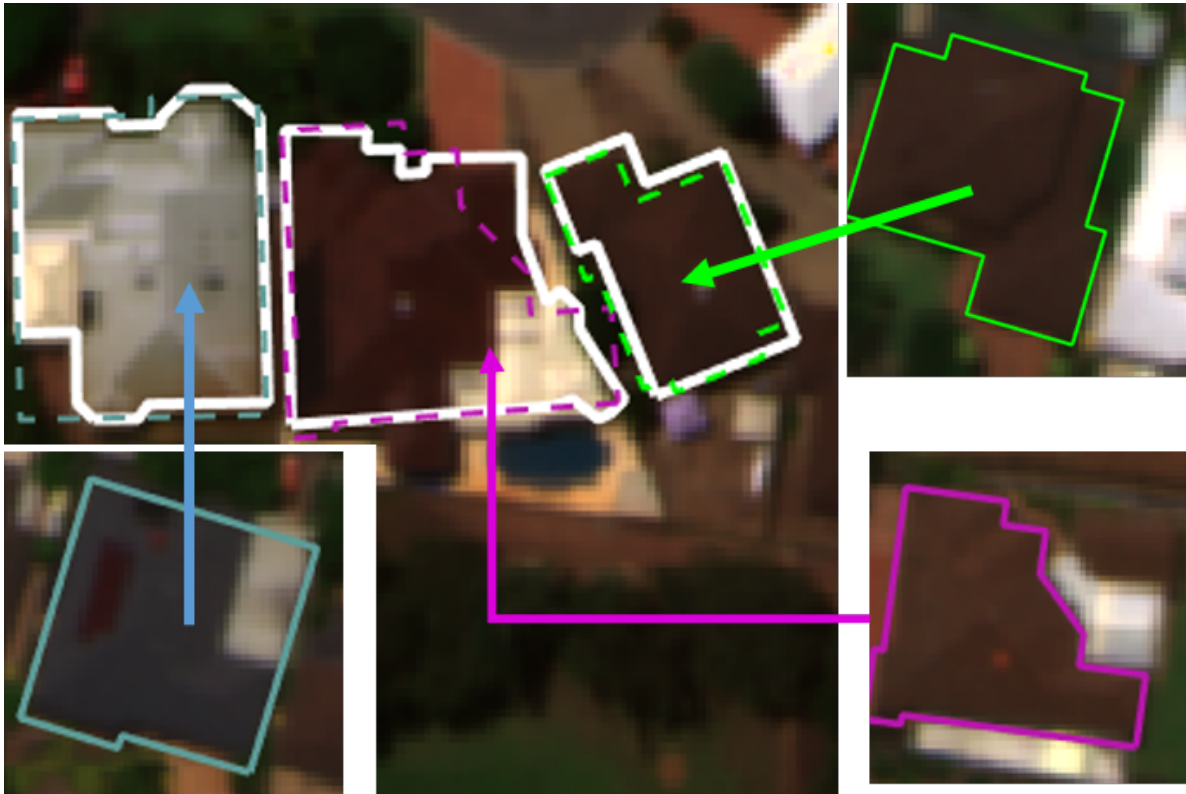
Figure 3. Examples of geo-typical building modeling. In three smaller image fragments, the library elements are depicted. The colors of their outlines coincide with their projections into the coordinate system of the multispectral image. For the left-most building pair, please note the difference in materials.
