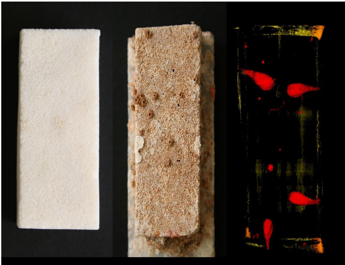
Figure 4.2 Experimental block of Porites lutea before and after 12 months of deployment, along with micro computerized tomography (microoCT) scan of the block post deployment. Varying sources of bioerosion displayed on the \mu\text{CT} image include grazing (orange), microboring (yellow), and macroboring by polychaetes and sipunculans (red)
