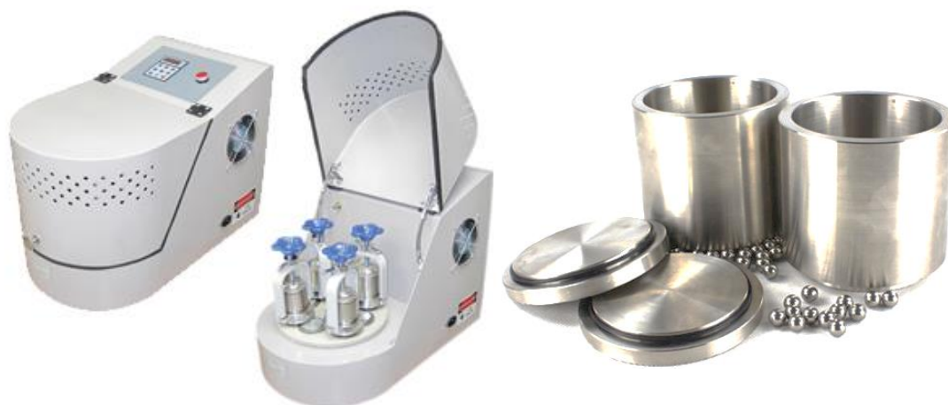
Figure 2.2 Picture of PQ-N04 planetary ball mill, canister and balls used for the synthesis. 3
