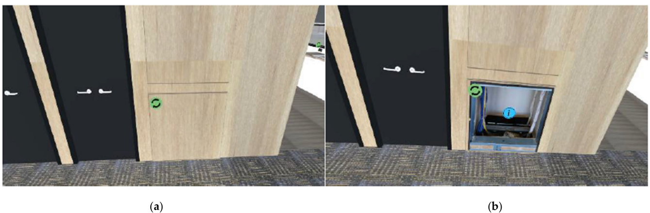
Figure 9. (a) Wall panelling hides the service duct connecting the roof space to the first floor and ground floor ceiling. (b) VR model exposes the lower access panel, revealing the service duct.
