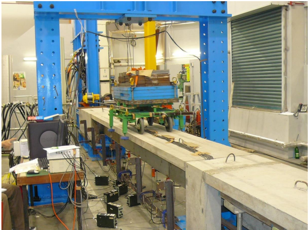
Figure 2-11. Overview of experimental setup of the bridge-vehicle system
