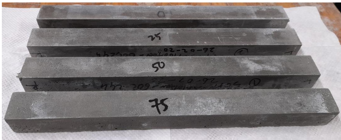
Fig. 7.5 The mortar prism bars after 1.5 years of immersion in \text{Na}_2\text{SO}_4 solution
