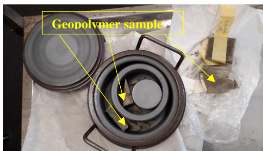
(a) Placing hardened geopolymer paste sample in the ring mill container
