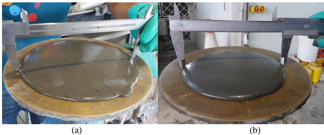
Fig. 4.1 Flow: (a) 100% fly ash (GFNS-0-B), (b) 75% GFNS with 25% fly ash (GFNS-75-B)
