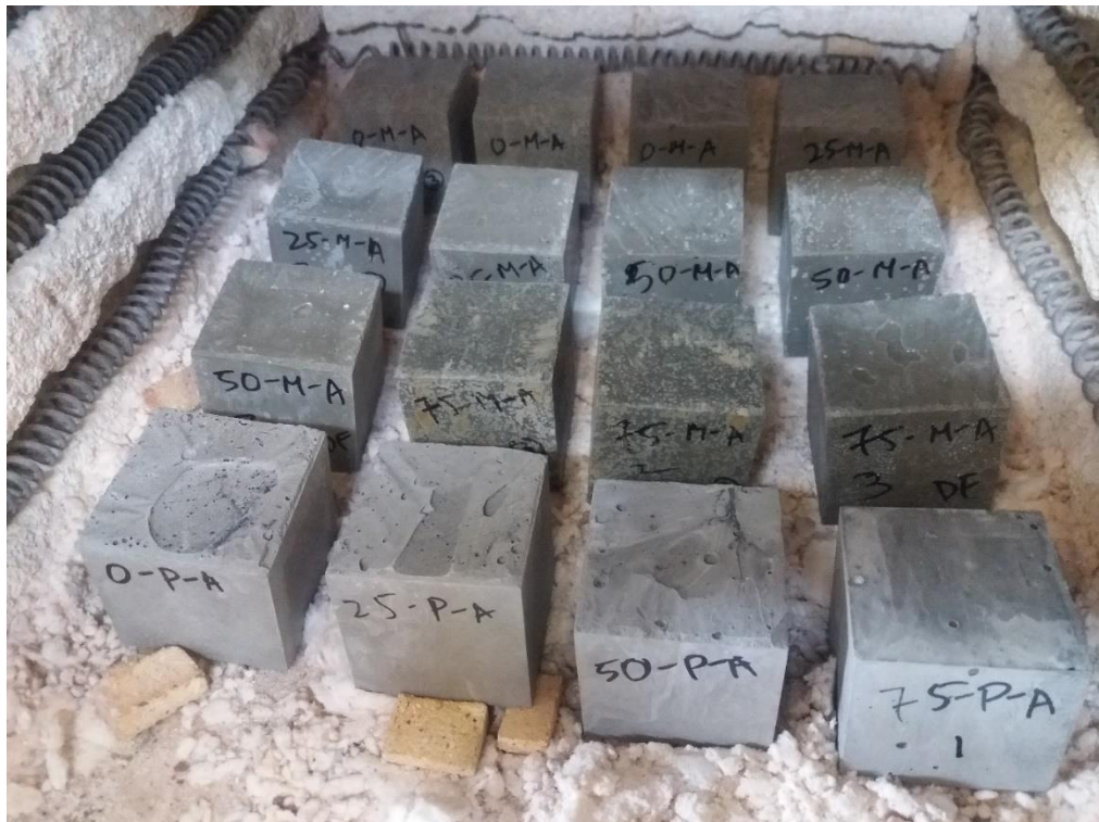
Fig. A.8 Elevated temperature exposure test
