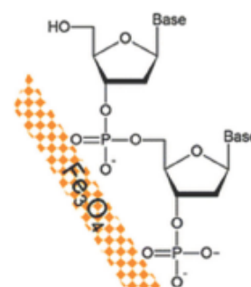
Figure 8. Two nucleotides in a single stranded DNA molecule where the \text{PO}_4^- interacts with magnetite ( \text{Fe}_3\text{O}_4 ), a common oxidation product of CS. This diagram was adapted from Liu and Liu (2014).
