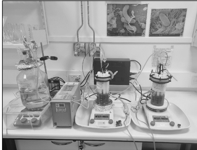
Figure 5: CDC reactor setup; with continuous flow for nutrient replenishment, maintained using an external reservoir attached to a peristaltic pump, replacing 30% of the reactor solution every 24 hours. Stirring hotplates were used to generate a constant temperature of 30°C and agitation at 50 rpm. Reactors were constantly flushed with pure N 2 gas to maintain anaerobic conditions.
