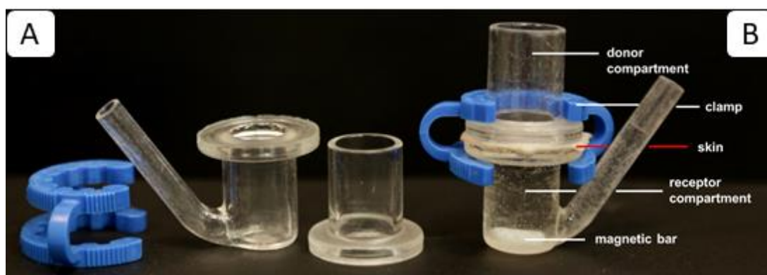
Figure 2.2 Franz diffusion cell set up: (A) disassembled (B) assembled cell
