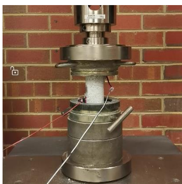
(a) Uniaxial compressive test
