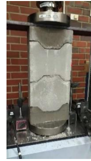
Figure 4. Compressive test setup for 2-block prism
