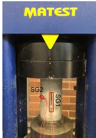
Figure 7-2. Quasi-static compression test setup (SG: strain gauge).
