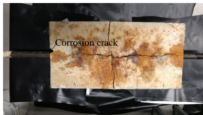
Figure 3.5: Specimen with corrosion crack.
