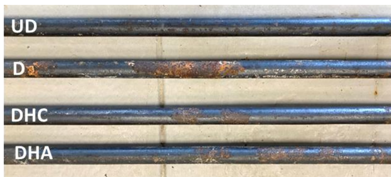
Figure 6.10. Visual inspection of rebar
