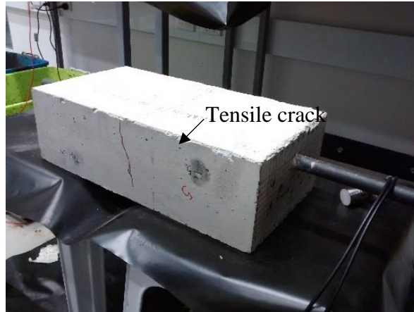
Figure 3.4: Specimen with tensile crack.
