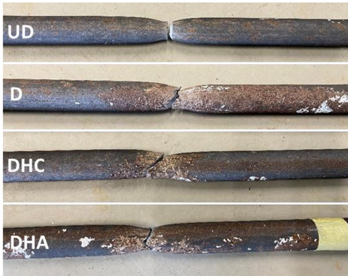
Figure 6.11. Fracture morphology for all specimens after tensile testing
