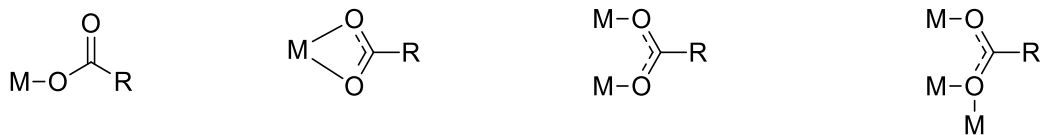
Figure 40: Coordination mode of carboxylate (from left to right): monodentate; bidentate; bridging; \mu_2\text{-}\eta^2,\eta^1 .
