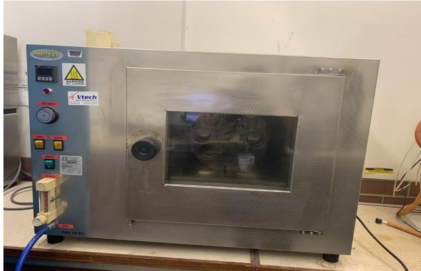
Figure 3.16: Apparatus of (RTFOT) tester, MATEST model at Curtin University
