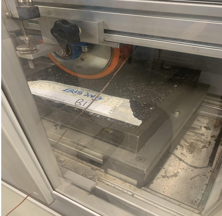
Figure 3.20: Wheel tracking sample and testing at Curtin University
