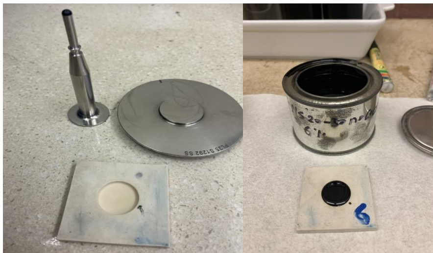
Figures 4.18: Show the plates of 25 mm and samples of PET-modified C320
