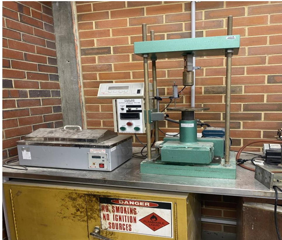
Figure 3.19: Marshall tests, OVILAB model
