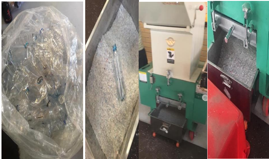
Figure 3.4: Waste plastic and grinding machine (photo by Nuha Mashaan)
