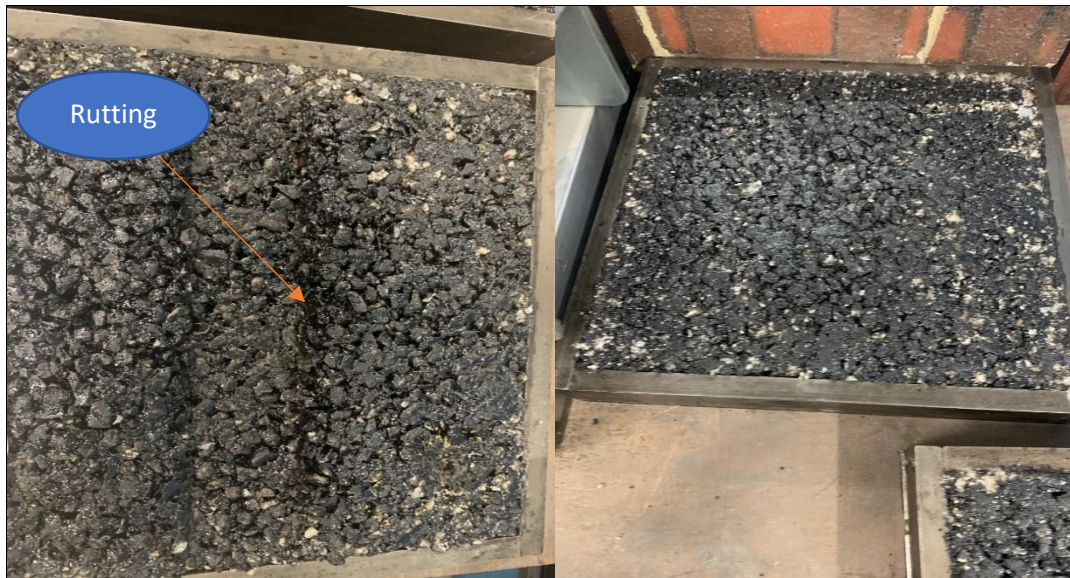
Figure 5.14: Rutting deformation for 0% PET (left) and 8% PET modified SMA (right)
