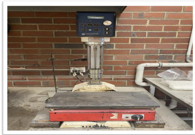
Figure 3.10: High shear mixer Silverson L5M-A used in binder preparation (photo by Mashaan)
