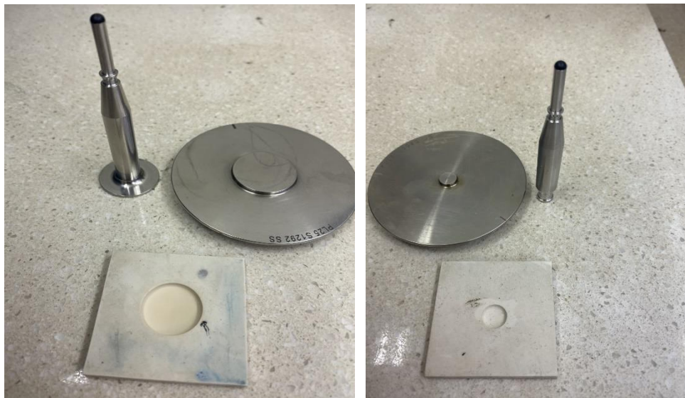
Figure 3.15: Plate and mould for unaged and RTFOT aged sample (left), plate and mould for PAV aged sample (right)
