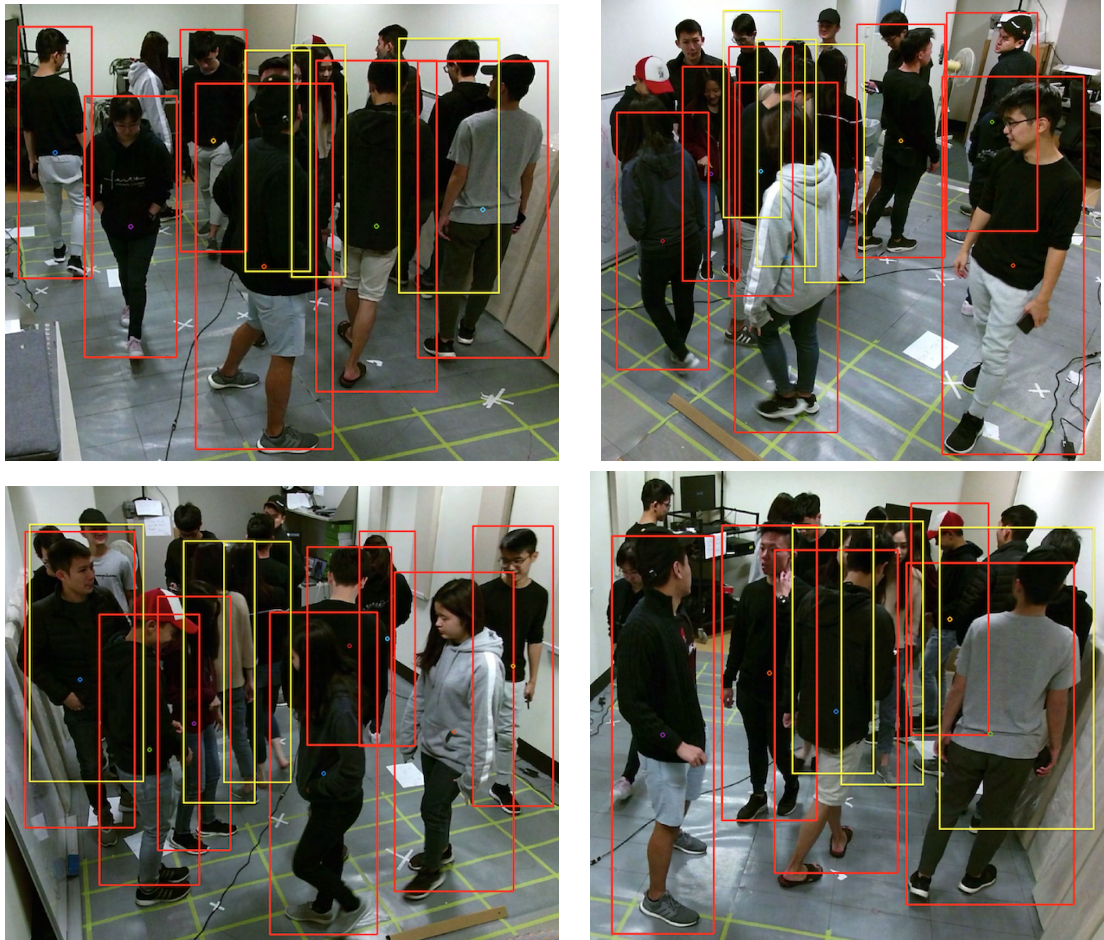
Figure 4.8: CMC3 Camera 1 to 4 (top left to bottom right): YOLOv3 detections (red bounding boxes) and people that are occluded in all four cameras (yellow bounding boxes).
