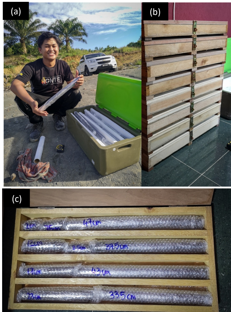
Figure 3.4: (a) Wrapped core sample in cushioned insulation box; (b, c) Core samples stored in coring boxes
