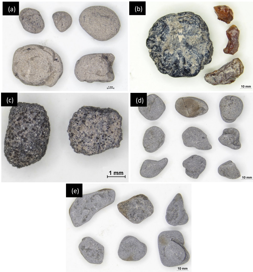
Figure 4.6: Closed-up photographs of some of the fragments retained in the drum (a) Miri Formation; (b) Tukai Formation; (c) Lambir Formation (d) Sibuti Formation; (e) Setap Shale Formation.
