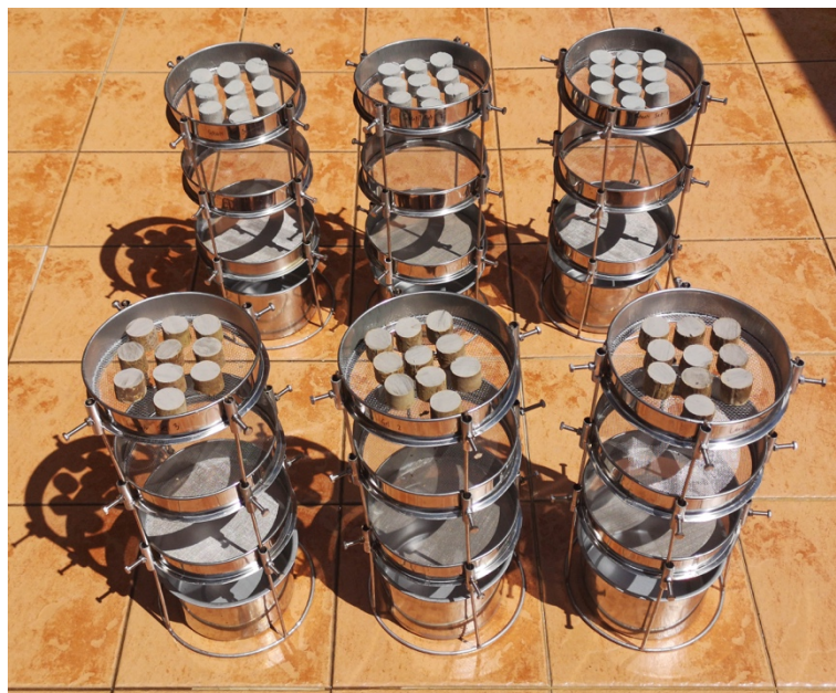
Figure 3.13: Natural slake test set-up exposed to the weather during the testing period.
