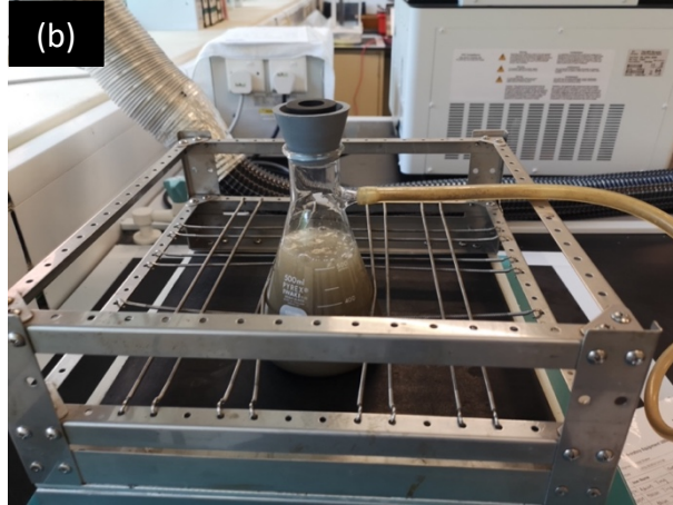
Figure 3.6: (a) Set up of the specific gravity test showing the volumetric flask (water pycnometer) connected to vacuum system and agitated in constant motion by using the orbital shaker. (b) Bubbles formed during deairing process to remove entrapped air in the slurry.
