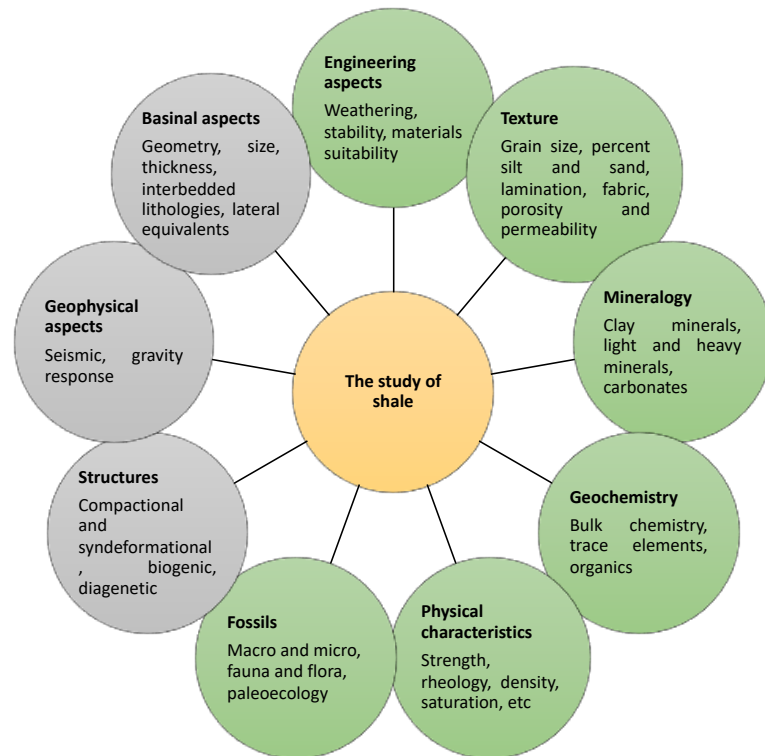
Figure 2.1: Typical approach contributing to the study of shale (modified after Potter et al. (1980))
