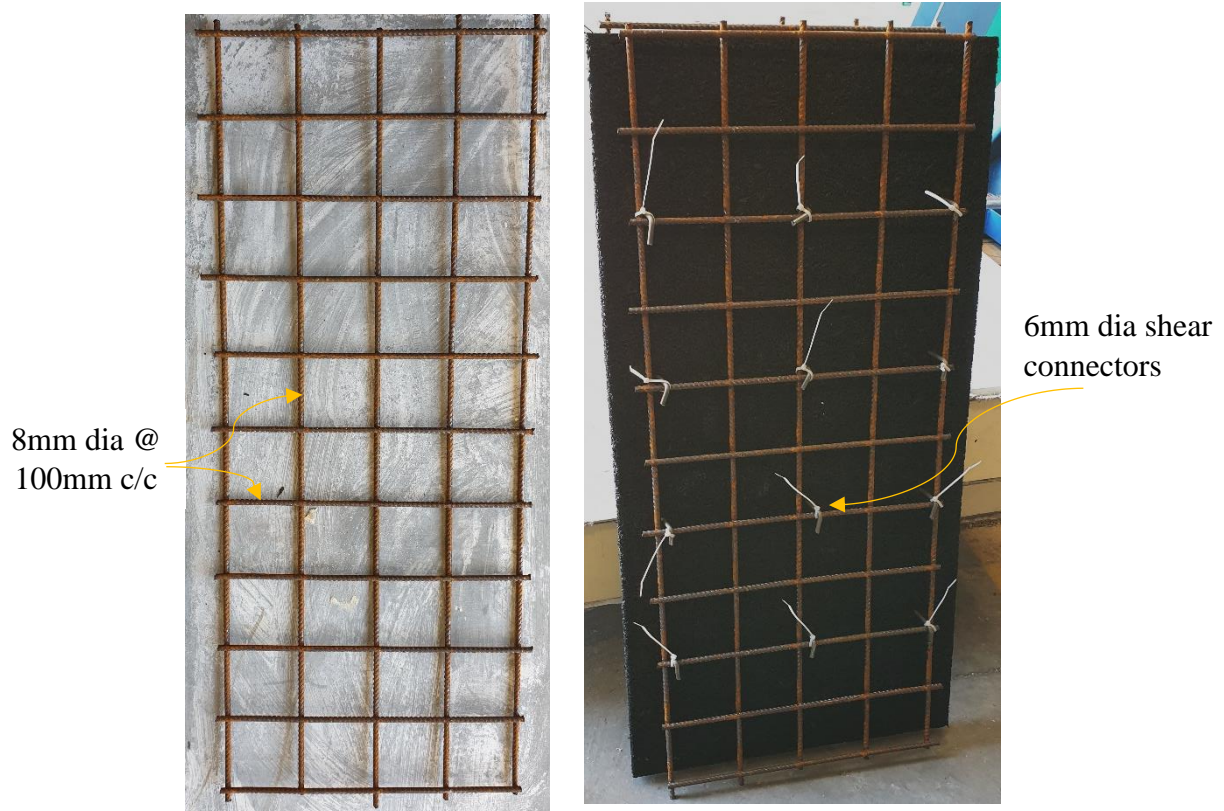
Figure 5-4 Steel mesh (SL81) and recycle tyre crumb rubber sheet with reinforcement details
