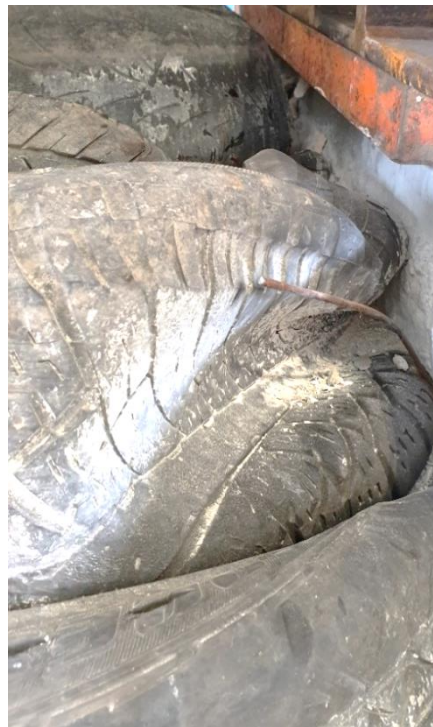
Figure 2-2 Cut steel wires in the tyre-bale simulating severe corrosion during service life
