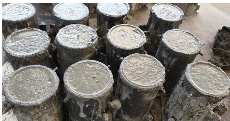
Figure 7-2 Concrete cylinder of SFRC taken at time of casting
