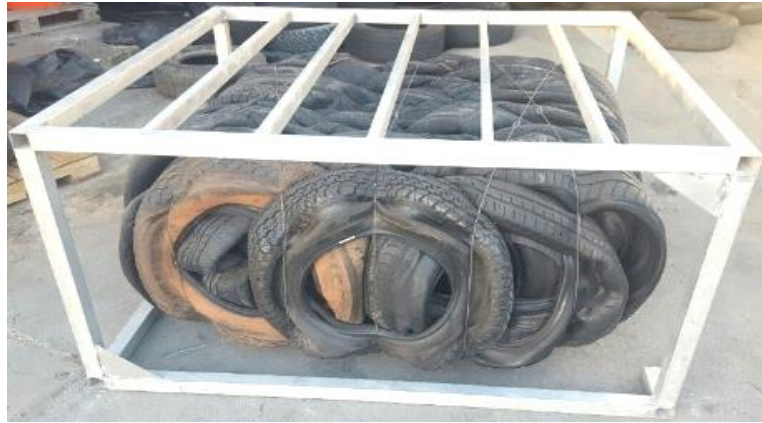
Figure 2-3 Typical tyre-bale made of used tyres
