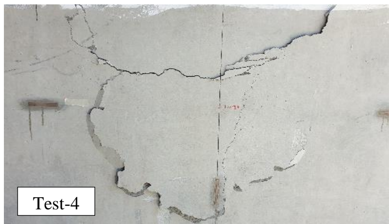
Figure 2-15 Failure behaviour in tyre-bale sandwich wall
