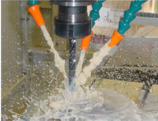
Fig. 8. Flooding with three nozzles.
