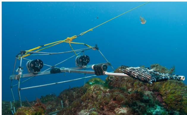
**FIGURE 1 |** Stereo BRUVS deployed *in situ*: a steel frame on which is mounted one or two video cameras (typically GoPro or small Sony camcorders) in underwater housings, in either a mono or stereo configuration. A container of bait is projected 1.5 m in front of the camera, attracting fish into the BRUVS video view. From Langlois et al. (2018).
