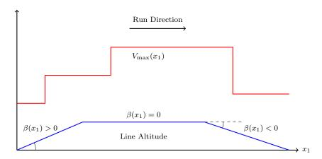
Figure 3. An example of a track with three line gradients and four speed limits.
