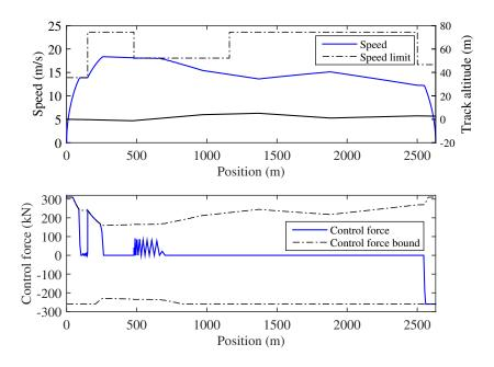
Figure 6. Optimal speed and control trajectories from Algorithm IV (T = 190 s).
