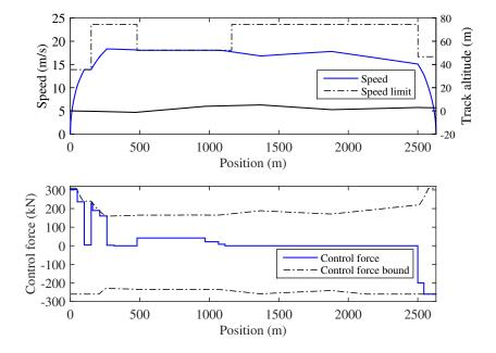
Figure 7. Optimal speed and control trajectories from Algorithm I (T = 170 s).
