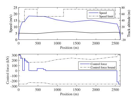
Figure 5. Optimal speed and control trajectories from Algorithm I (T = 190 s).
