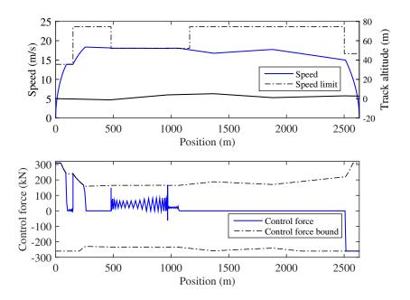
Figure 8. Optimal speed and control trajectories from Algorithm IV (T = 170 s).
