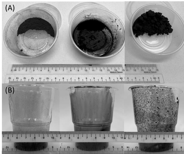
Figure 3.11: (A) Physical Conditions of 0.175g Nanofiller (B) Liquid Phase of OPEFB Nanofiller Composite Mixtures (Left: Nanoplatelets, Middle: Nanopowder, Right: Nanotube < 30nm)
