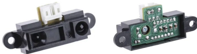
Figure 7.8: Reflective sensor (GP2Y0A41SK0F, Sharp)
