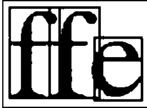
Figure 5.14: Overlapping of ideal bounding boxes due to the shapes and placement of characters in the ideal document.
