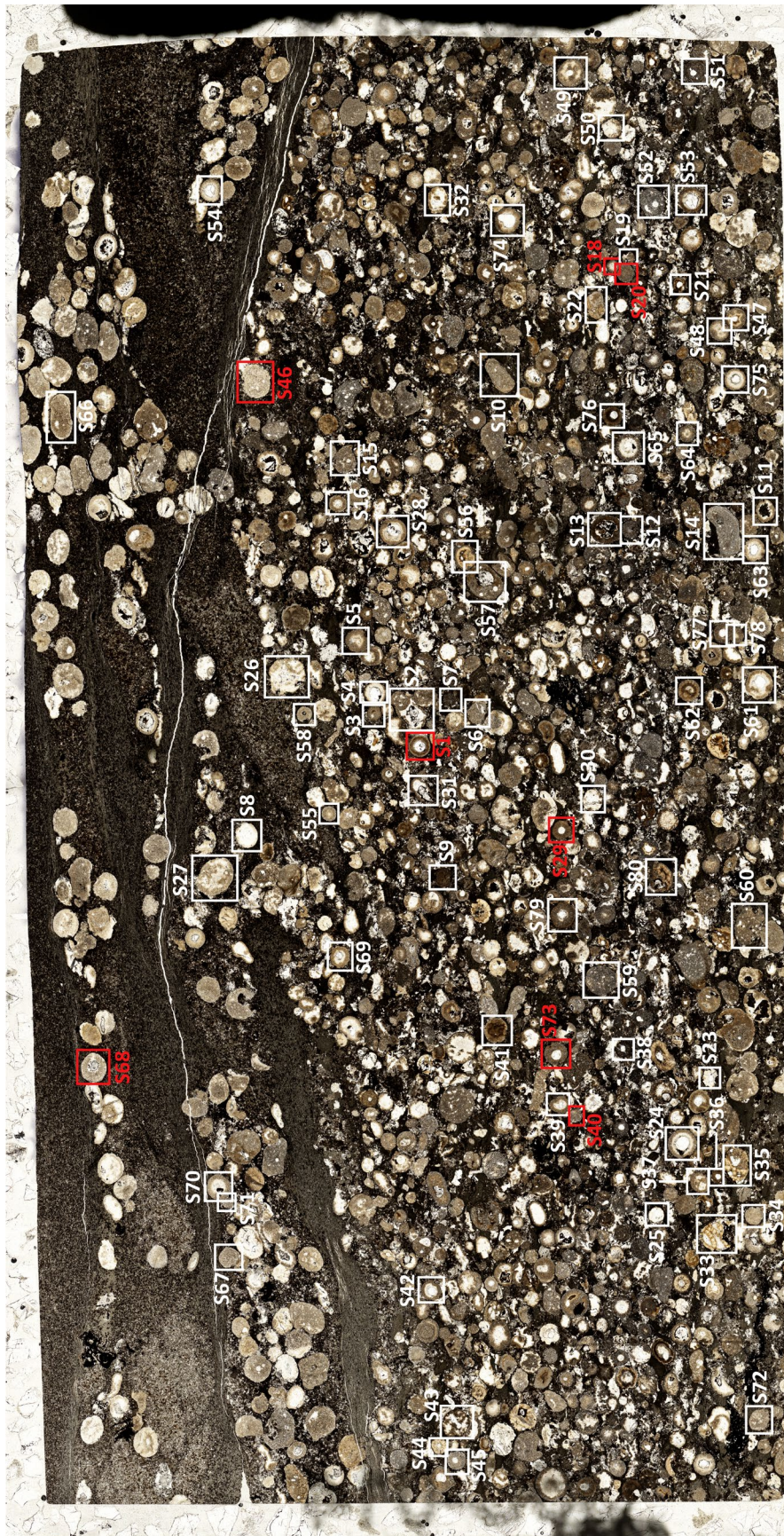
PPL navigation map for thin section BGS L-1/BGTS for Bee Gorge spherule investigations, red annotations represent EBSD examined spherules (n=18).
