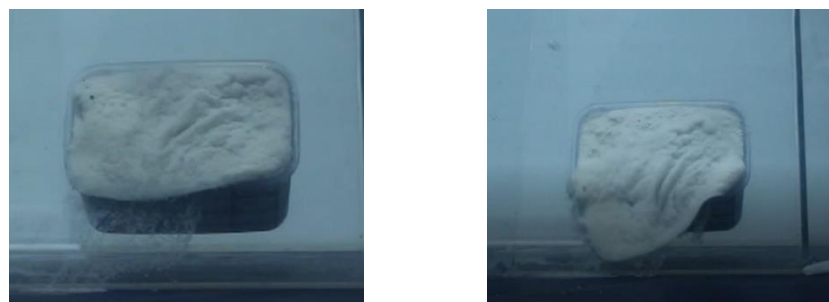
Figure 7.5 Photographs of the dislodging sheet-like biopolymerised layer.
