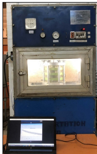
Figure 5. Triaxial test for resilient modulus.
