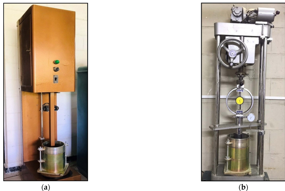
Figure 4. The CBR test. (a) Specimen compaction. (b) CBR testing.
