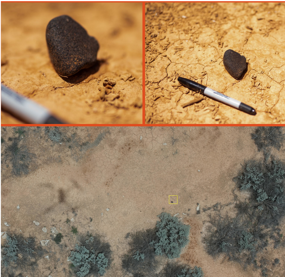
Figure 4. The recovered meteorite as seen in person (top two panels), and from the survey drone (bottom panel). For scale, a 15 cm long felt pen is placed next to the meteorite (top right). The yellow box in the bottom image is 22 cm on one side.
