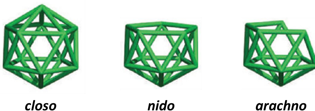
Figure 1.13. The three most common classes of borane structures: closo -boranes, as in B_{12}H_{12}^{2-} , nido -boranes, as in B_{11}H_{13}^{2-} , and arachno -boranes, as in B_{10}H_{15}^{-} . Reproduced and adapted with permission. [48]. Copyright 2009, Springer Nature.
