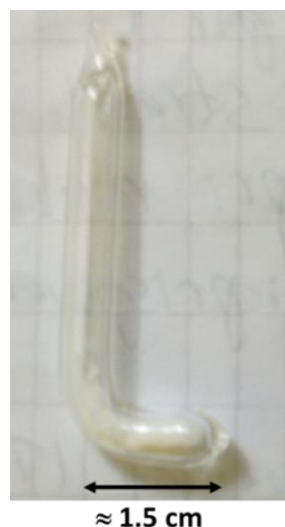
Figure 2.4 'L-shaped' quartz NMR tube containing \approx 40 mg of sample used to investigate the ^{11}\text{B} spin-lattice NMR relaxation rates.
