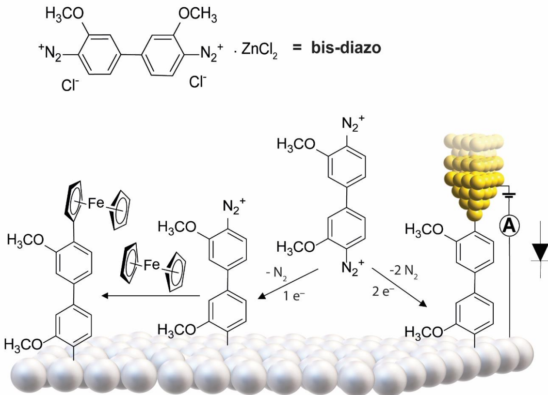
Figure 1. Structure of the molecule ( bis-diazo ) studied and a schematic describing its reaction with surface and tip electrodes or with ferrocene. The surface and tip electrodes can be gold or silicon.
