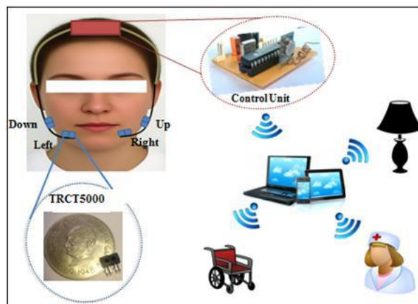
Figure 10: System architecture- wearable tongue controlled assistive device [23]
