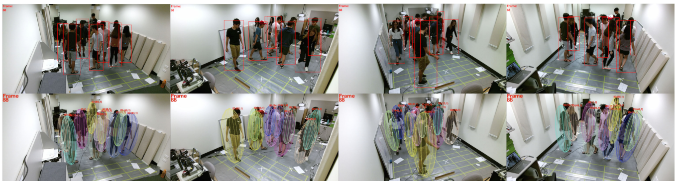
Fig. 7. CMC2 Camera 1 to 4 (left to right): YOLOv3 detections (top row) and MV-GLMB-OC estimates (bottom row).
