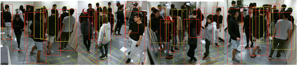
Fig. 8. CMC3 Camera 1 to 4 (left to right): YOLOv3 detections (red bounding boxes) and people that are occluded in all four cameras (yellow bounding boxes).
