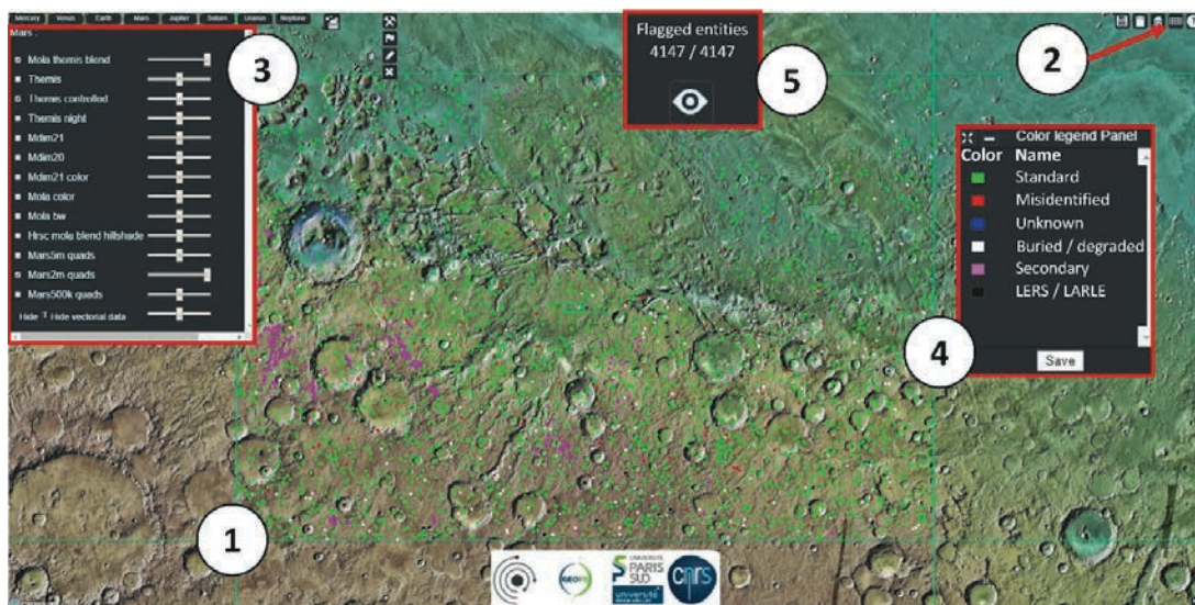
Figure 2. Principal functionalities of the interface: (1) Mars 2M quads corresponding to the division of the database, the limit of quadrangles considered in this study; (2) projection mode (planisphere or globe); (3) data panel allowing display of one or more data set with transparency level; (4) legend panel grouping the four main categories as well as flagging uncertain and misidentified entries; (5) number of displayed impact craters and number of displayed impact craters that are already classified. Each colored dot corresponds to an impact crater in the Robbins and Hynes (2012) database.
