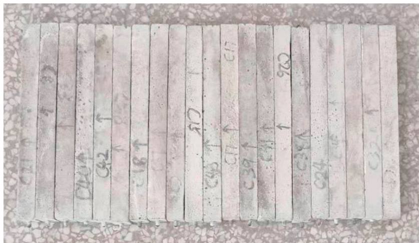
Fig. 3 – Bar samples for ASR expansion test.
