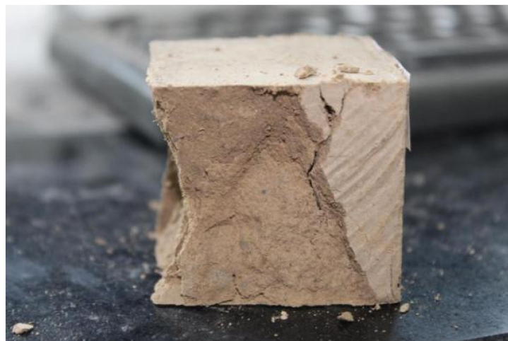
Figure 7. Fracture surface of conventional CSS sample.
