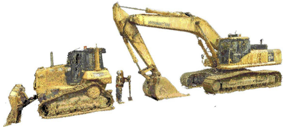
Figure 5. Hazardous situation of worker and equipment measured by a 3D laser scanner [66].
