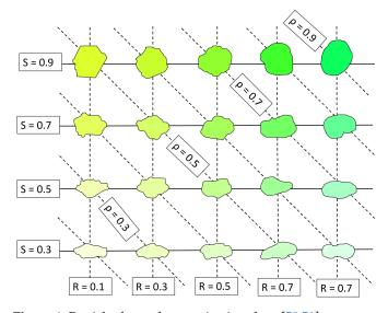
**Figure 4.** Particle shape characterization chart [50,51].
