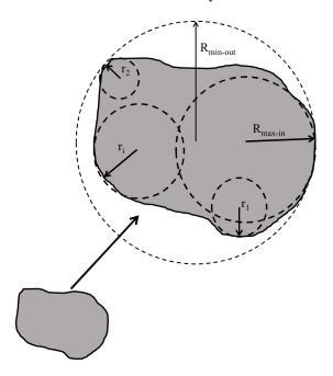
Figure 3. Particle shape parameters used in defining roundness [50,51].
