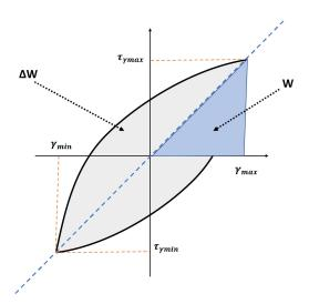
Figure 6. Hysteresis loop in cyclic tests.
