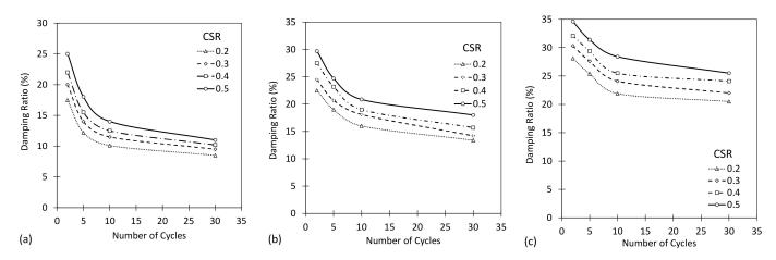
**Figure 8.** Effects of increasing number of loading cycles on the damping ratio for different CSR conditions and vertical stresses of (a) 50 kPa, (b) 150 kPa and (c) 250 kPa for the first reconstruction.
