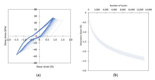
**Figure 7.** Results of the cyclic tests for CSR = 0.3 and vertical stress = 150 kPa: (a) shear stress–strain hysteresis loops; and (b) volumetric strain by number of cycles.
