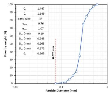
Figure 1. Grain-size distribution curve of the test sand.
