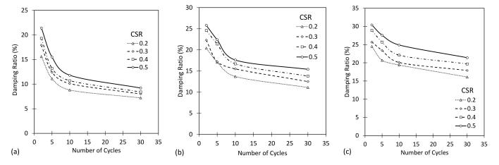
**Figure 9.** Effects of increasing number of loading cycles on the damping ratio for different CSR conditions and vertical stresses of (**a**) 50 kPa, (**b**) 150 kPa and (**c**) 250 kPa for the second reconstruction.
