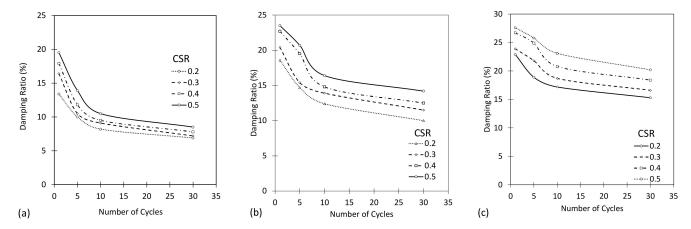
**Figure 10.** Effects of increasing number of loading cycles on the damping ratio for different CSR conditions and vertical stresses of (a) 50 kPa, (b) 150 kPa and (c) 250 kPa for the fifth reconstruction.
