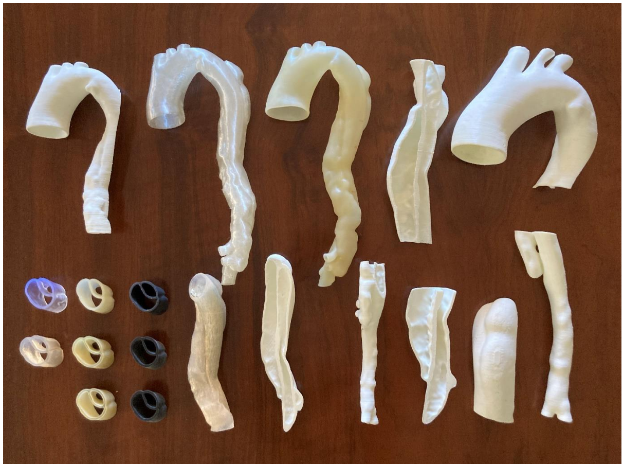
Figure 2.5 To test mechanical and radiological properties, models were printed through different printing materials.
