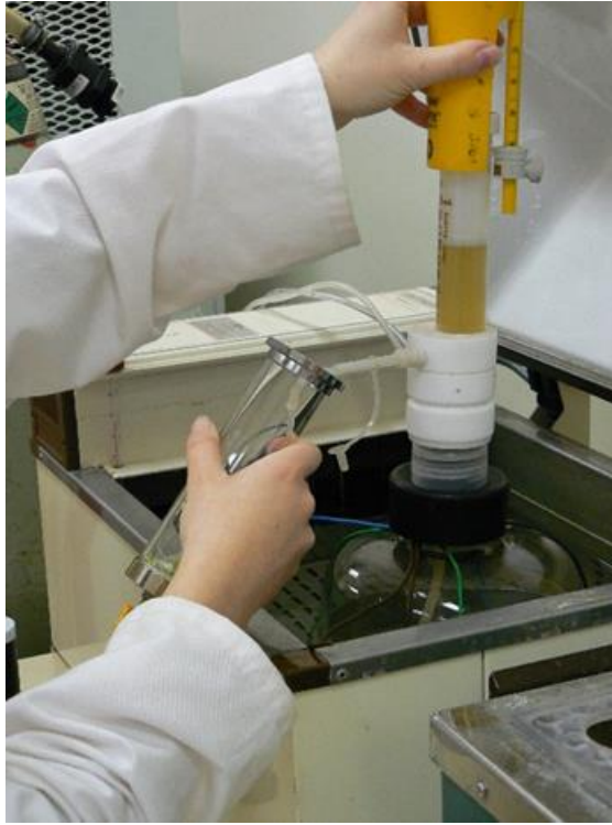
Figure 3.3: Filling the glass syringes with buffer solution using the bottle top dispenser (courtesy C. von Pirch)
