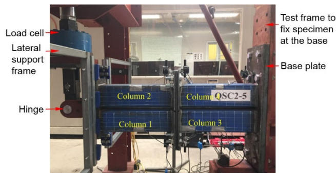
668 669 Fig. 21. Connection test which adopts the stub column assembly for a modular connection incorporating resilient layers [35].
