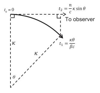
FIG. 6. Sketch of the time delays associated with synchrotron radiation. At time  $t_0 = 0$  a particle is oriented towards an observer. After subtending an angle  $\theta$  with curvature radius  $\kappa$  at velocity  $v = \beta c$ , it is time  $t_1 = \kappa \theta (\beta c)^{-1}$ . Radiation emitted at time  $t_0$  takes a time  $t_2 = (n/c)\kappa \sin \theta$  to be equidistant to the observer.
