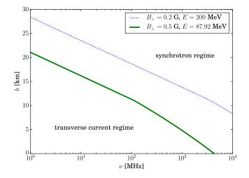
FIG. 8. Height *h* in the atmosphere at which  $\ell'_{\text{synch}} = \chi_0$ , computed for two combinations of magnetic field/electron energy. Above this height is the synchrotron regime where  $\ell'_{\text{synch}} < \chi_0$ , and below this the transverse-current regime, where  $\ell'_{\text{synch}} > \chi_0$ .
