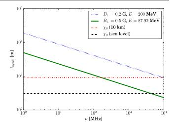
FIG. 7. Characteristic length scale  $\ell_{\text{synch}}$  over which  $e^{\pm}$  synchrotron radiation is observed for an observer in the plane of the emission. This is computed for two combinations of perpendicular magnetic field  $B_{\perp}$  and electron energy E, and compared to the radiation length  $\chi_0$  at two different altitudes.
